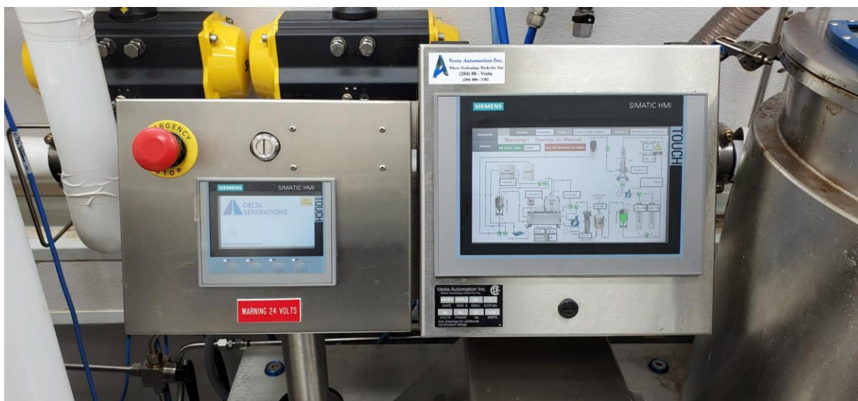
Figure 4 – extractX-developed HMI panel used to direct and control the automated extraction process
